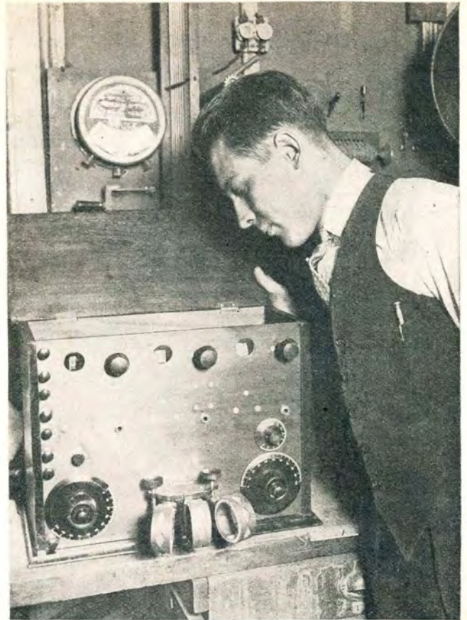
M. W. Obermuller's receiver utilizes three stages of transformer coupled radio frequency, detector and two stages of audio frequency. It has but one control, aside from the rheostats and one potentiometer. The efficient workmanship is probably responsible for the fact that Mr. Obermuller has brought in stations far distant and no squeals are encountered in tuning. (K. & H. Photo)
